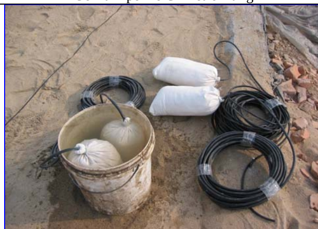
长效硫酸铜参比电极 Permanent Cu/CuSO 4 Reference Cell
