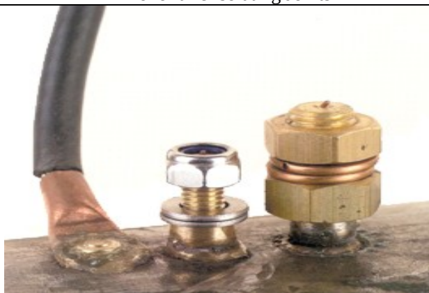
测试电缆连接用铜焊机、焊钉 Pin Brazing Unit and Pins
